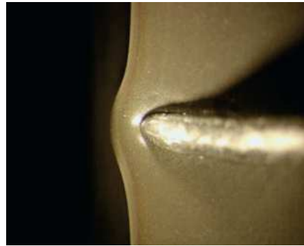
The sealing lips of a Simmerring, following a test cycle with a standard FKM material (above, with crack formation when lifting) and a BRE-FKM material 75 FKM 260507.
