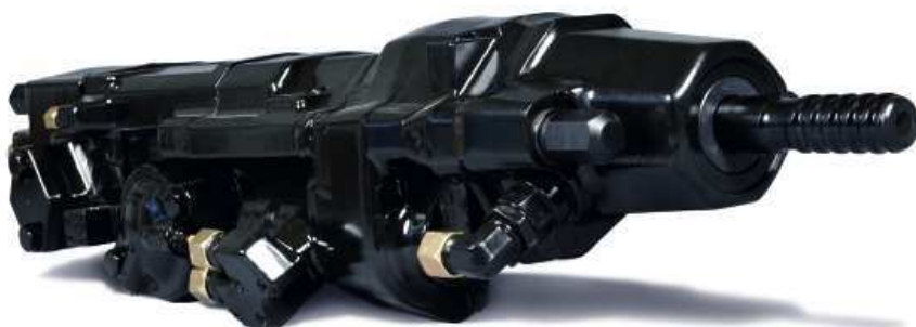
COP 3038 hydraulic rock drill: highest requirements for seals
